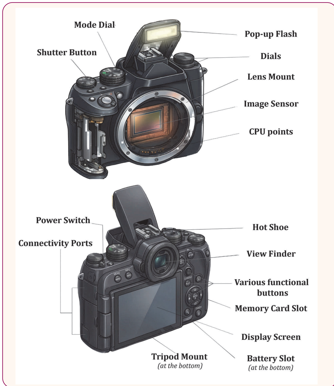
Fig. 2.4.5. Parts of a Camera Body
